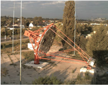
(b) Single-mirror MST prototype in DESY Berlin.
